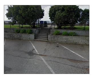
The new parking layout provides a hatched 1.3 metre path to access the Promenade stairs. Given that the stairs themselves are not wheelchair accessible, this path should be wide enough for those wishing to access the Promenade at the various stair locations.
