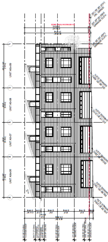
1 BLOCK 2 - EAST ELEVATION 1/8" = 1'-0"
