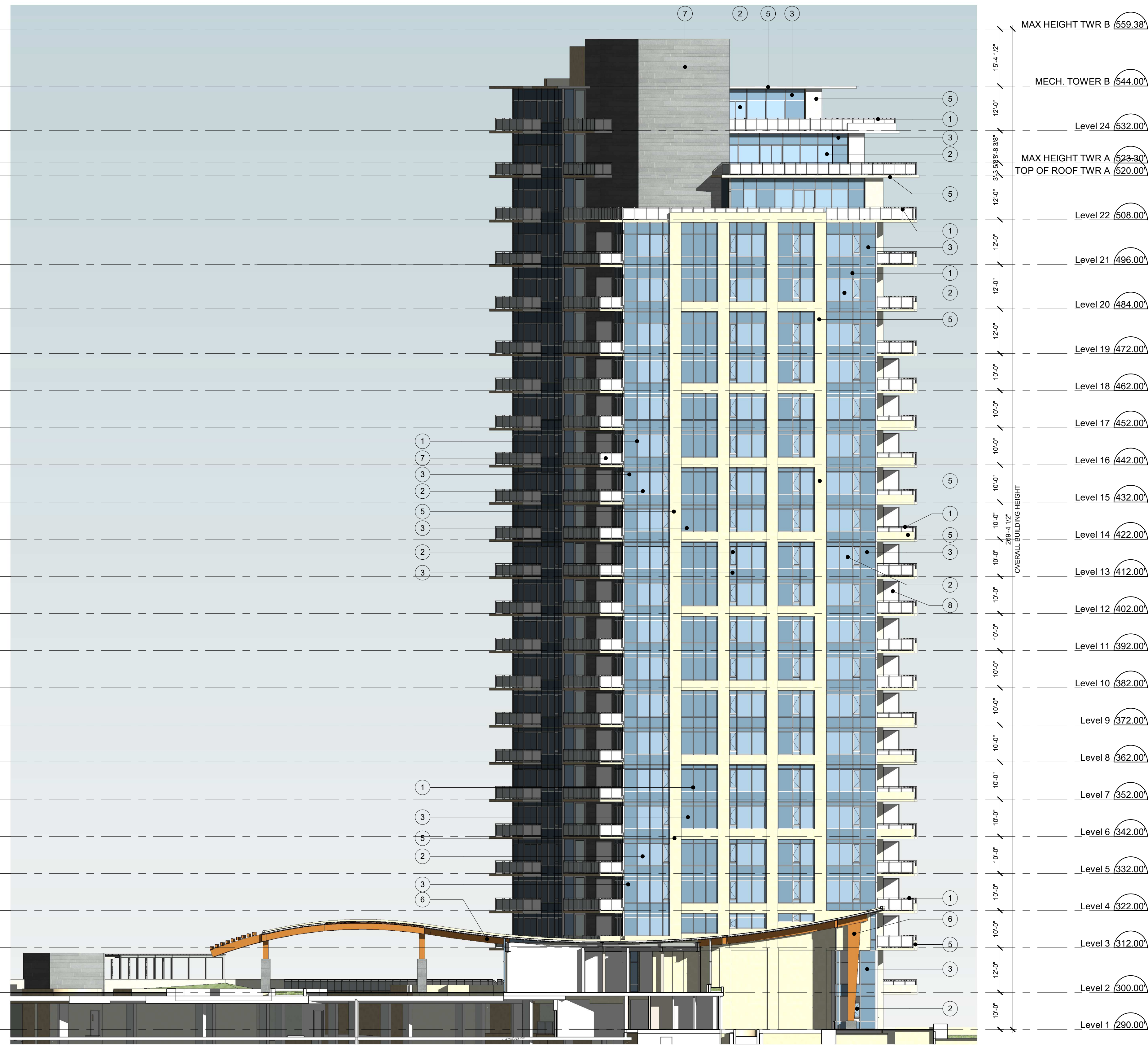
2 Tower B NW Elevation (DP) 1/16" = 1'-0"
