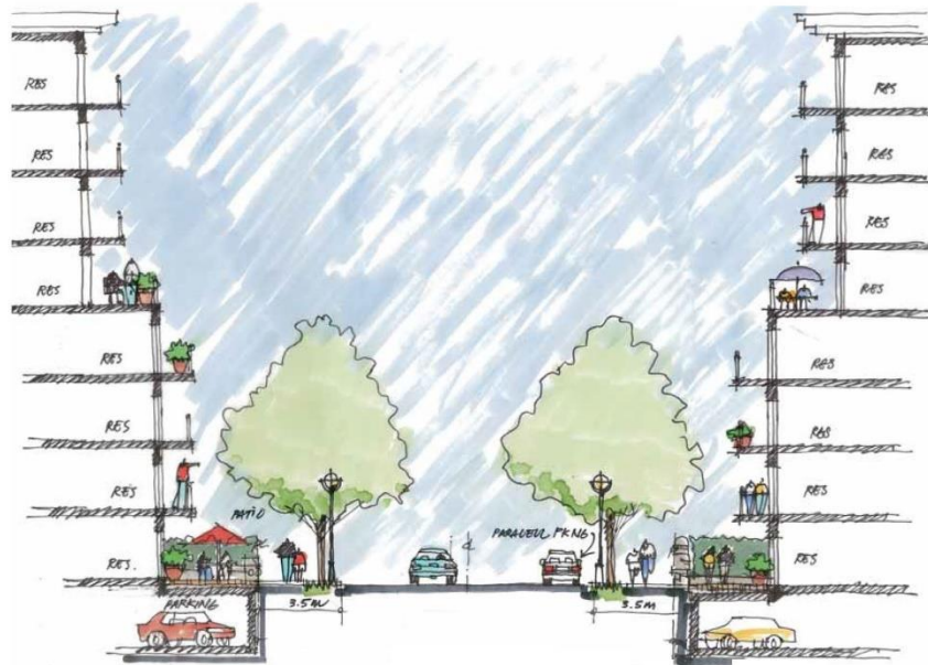
Section showing residential step-backs, parking, pedestrian realm and use of street fronting outdoor amenity spaces.
