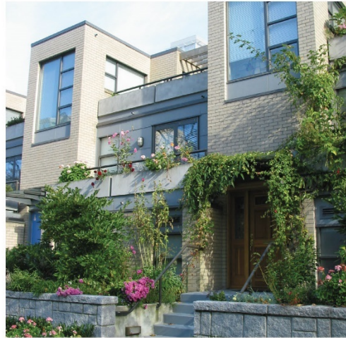
Guidelines c and i: Massing and natural materials are varied to break up the building front and create visual interest
