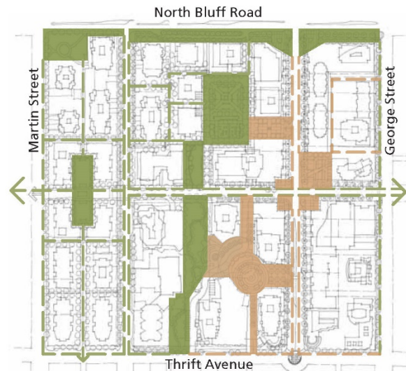
Guidelines b and f: Building siting creates a fine-grained network of pathways, parks, and open spaces
