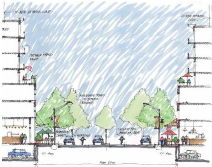
Diagram showing illustrative example of mixed-use building step-backs and pedestrian realm along Johnston Road
