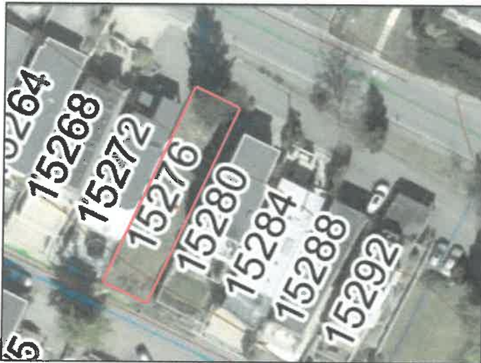
Figure 1. Aerial photograph from WROMS of the site at 15276 Columbia Avenue with water (blue), storm (green) and sanitary (red) located in the lane off the south side of the lot.
