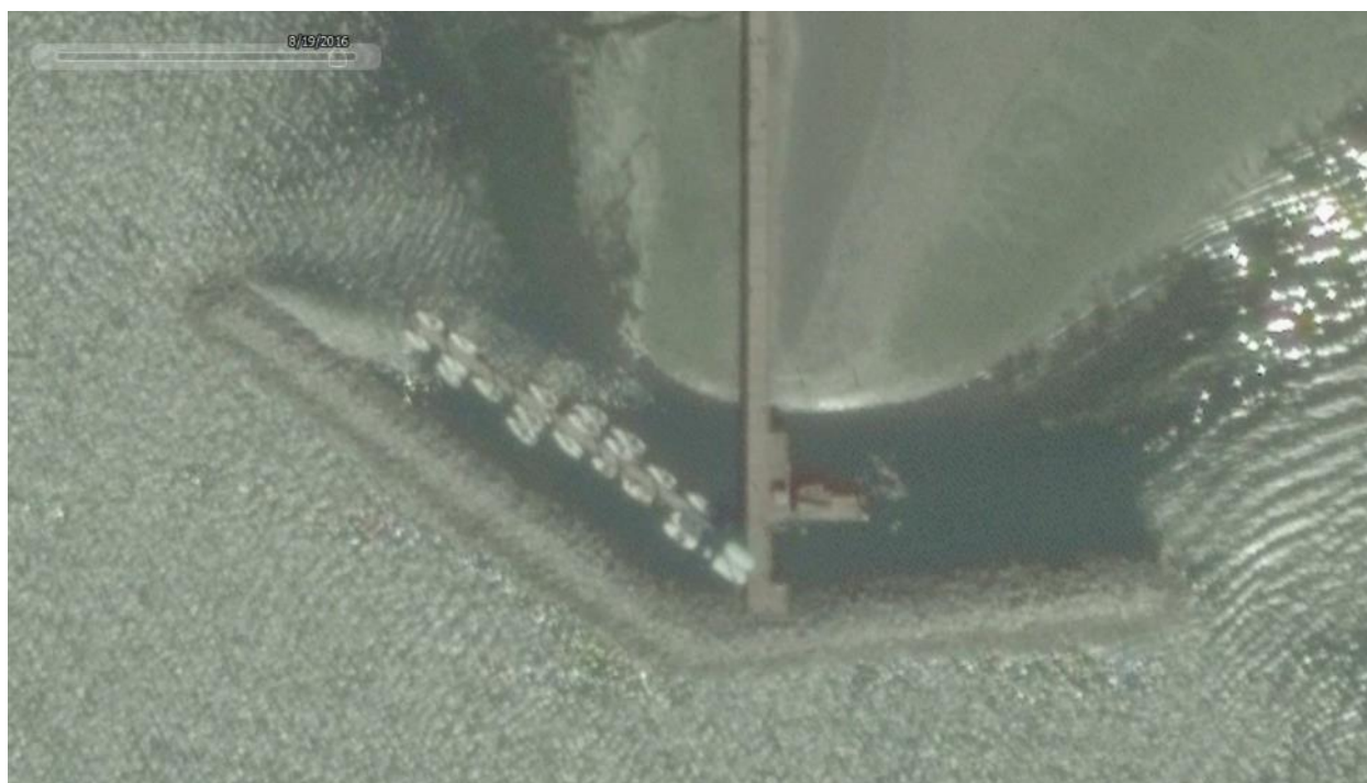
Figure B View of Waves Refracting Around West End of Breakwater.
