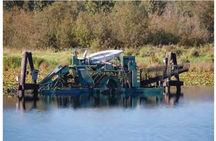
Harvester used to remove aquatic plants from the surface of Burnaby Lake
