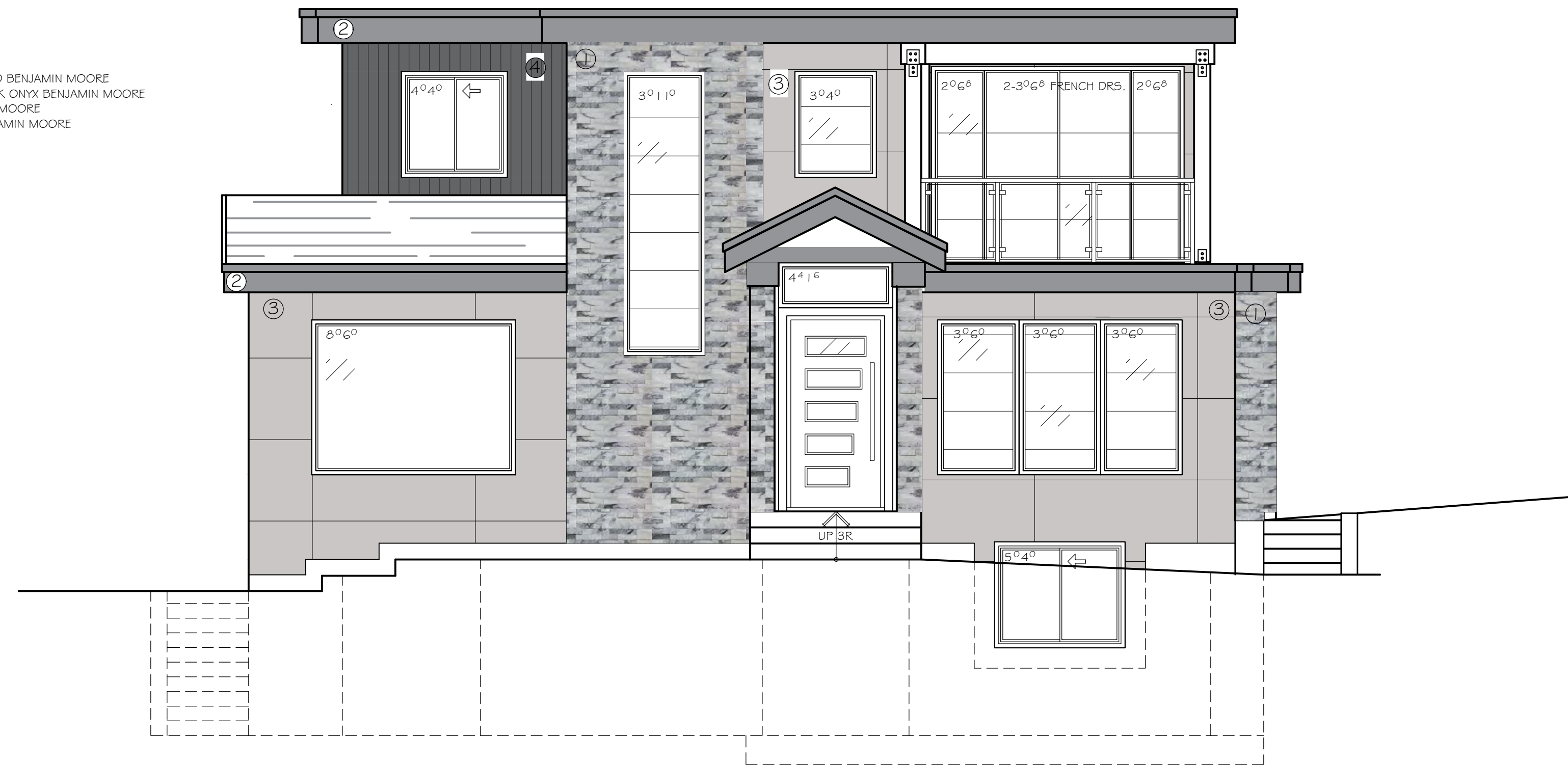
UNIT 'A' LEFT ELEVATION (EAST) SCALE: 1/4" = 1'
