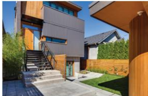
Guideline 22.8.2 (i), On-site parking using pervious materials.
