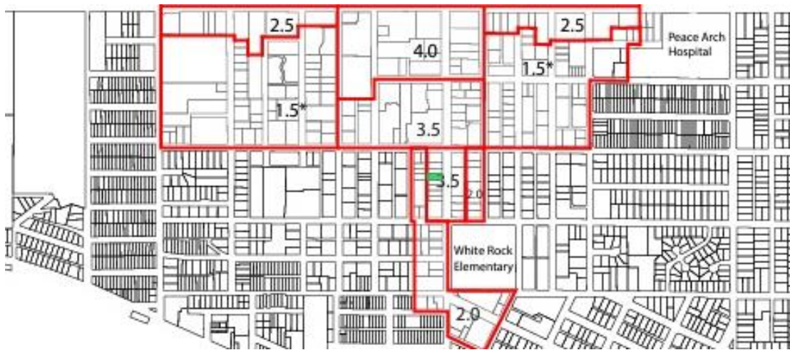
Figure 1: Maximum FAR in the Town Centre, Town Centre Transition, and Lower Town Centre Areas (Figure 9 in OCP). The Parcel highlighted in green is the subject site.
